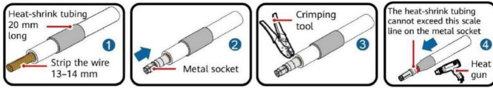
Figure 4-7 Connecting DC output cables and signal cables
