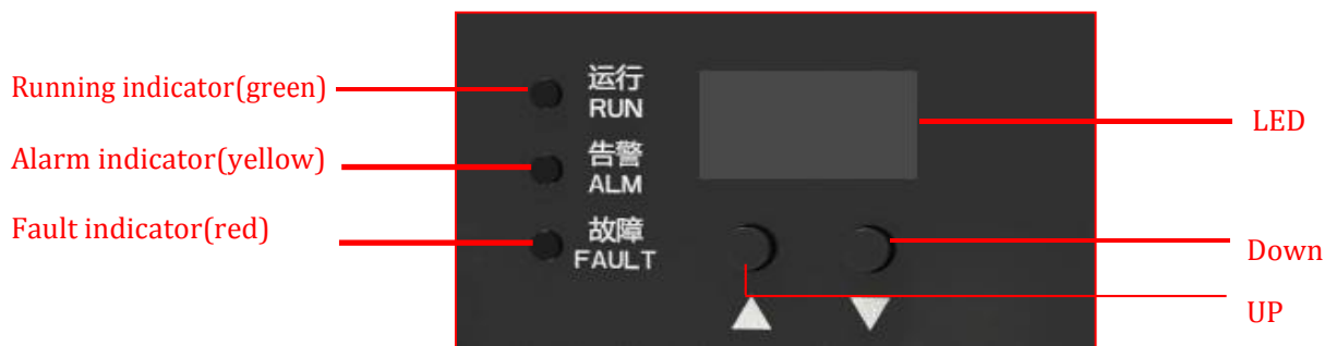
Figure 2-2 front panel Schematic diagram
